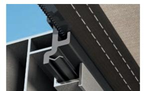
**OptiStretch or Stretch – for a stable fabric position** With Plaza Viva OptiStretch the fabric is held captive and on all four sides. The advantages: a highly tensioned fabric and no light gap on the sides. The basic version of the Plaza Viva Stretch is tensioned on two sides and there is a light gap between the fabric and guide channel. A strong rope tensioning system ensures even fabric positioning with both versions.
